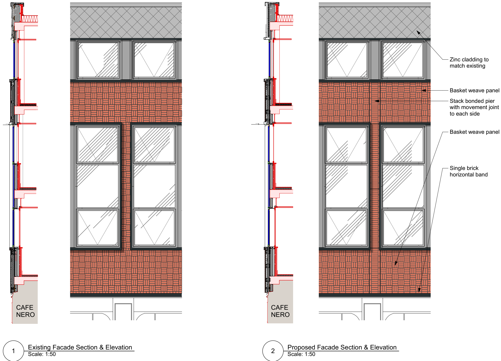
Figure 6 Extract from HFM drawing P301 - showing existing and proposed cladding bay's side by side.
