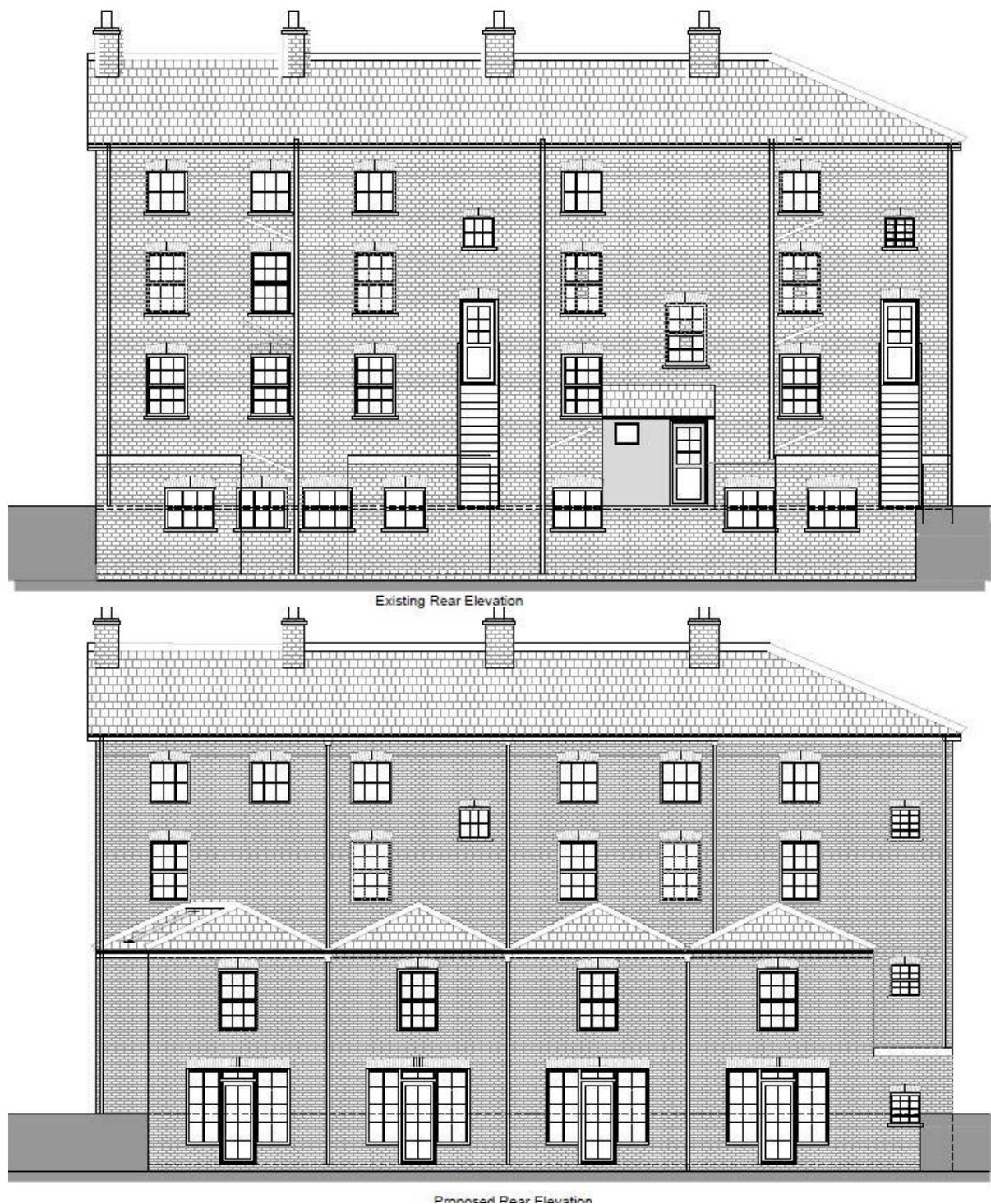
Figure 6: Existing and Proposed rear (North) Facades
