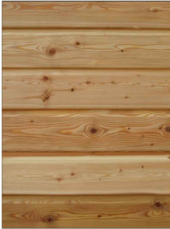
Fig. 2 Photograph of timber cladding to be used. Specification: Siberian larch shiplap cladding
