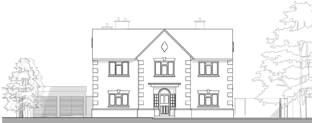
Existing street elevation, showing garage clad in exposed aggregate plastered panels, at odds with the brick building.
