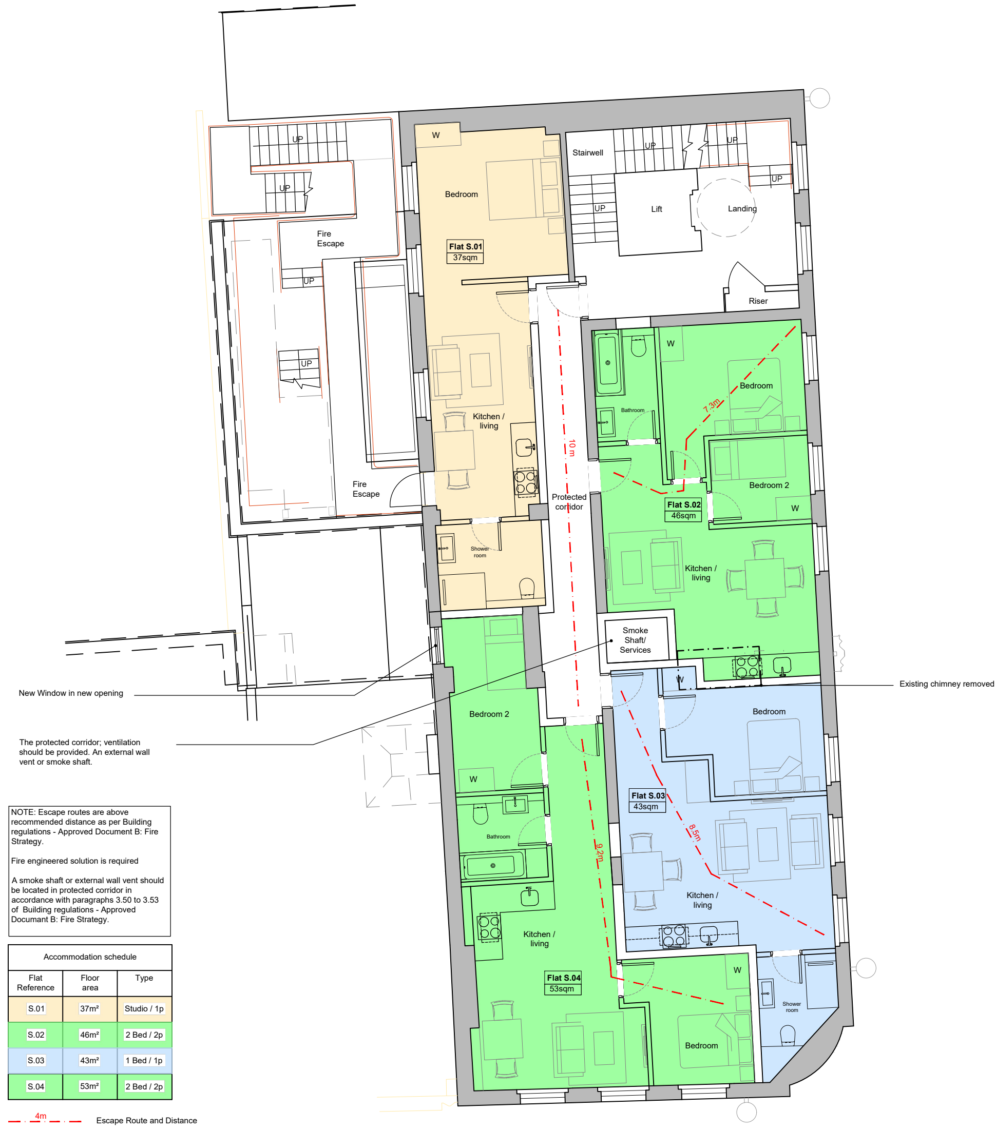
1 Station Road - Additional Windows 2nd Floor Plan
