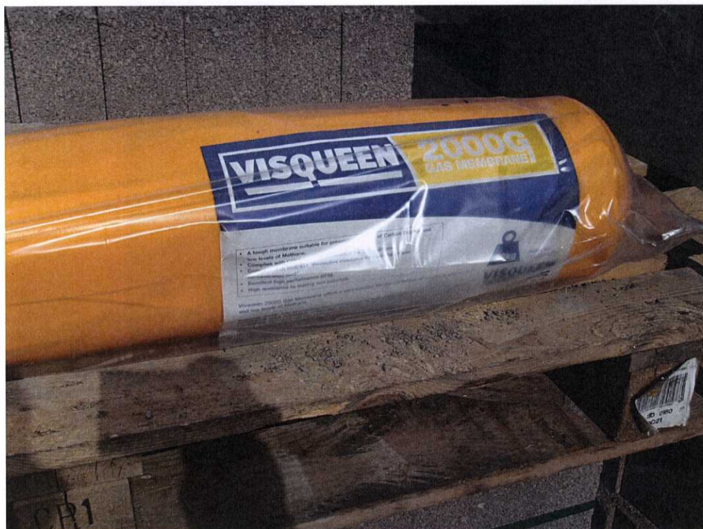
Materials used in Landgas Mitigation Measures- 20 th May 2009
