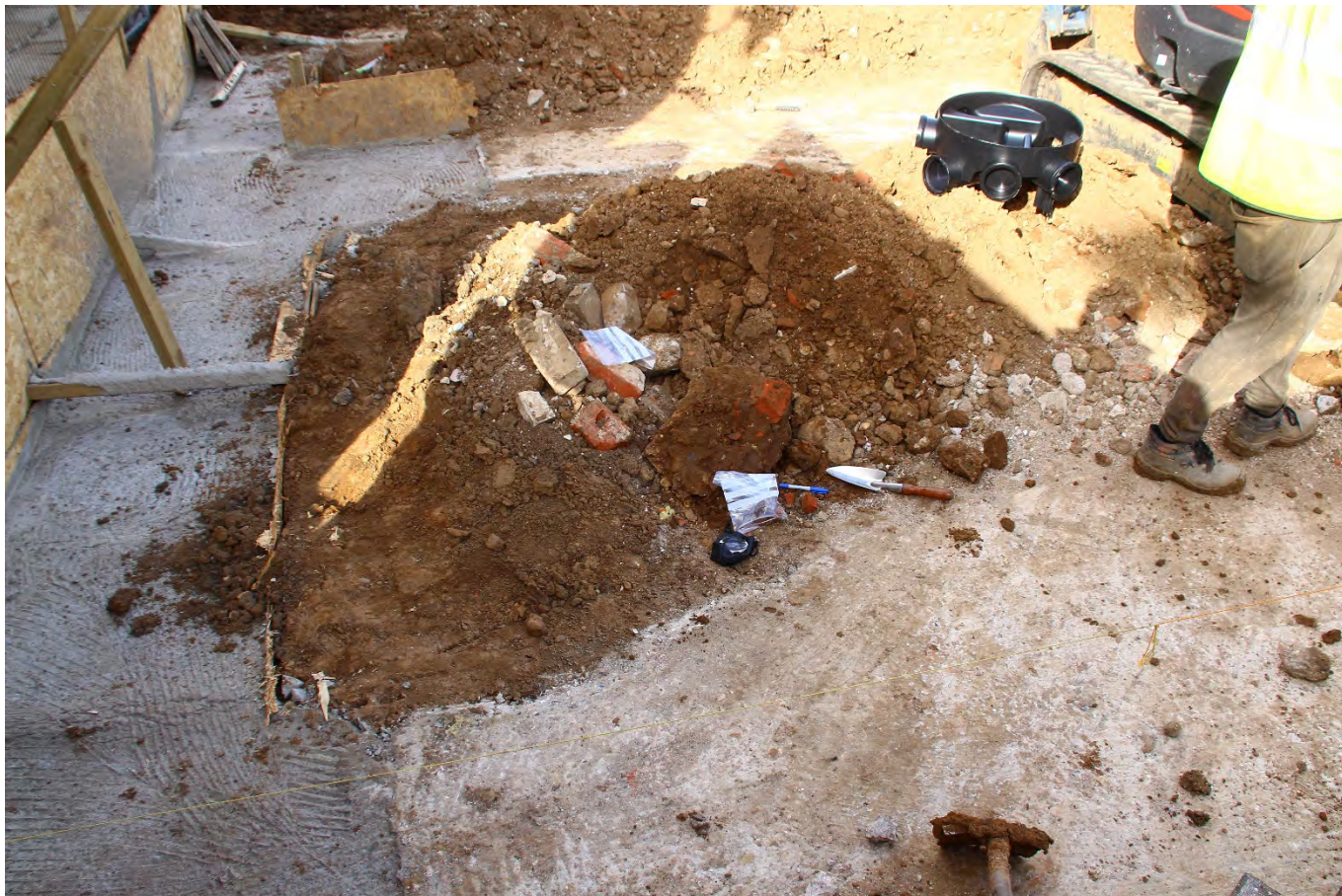
Above and below, re-examination and sampling of the remains of the overlying soils in the borehole BH8 and oil spillage location
