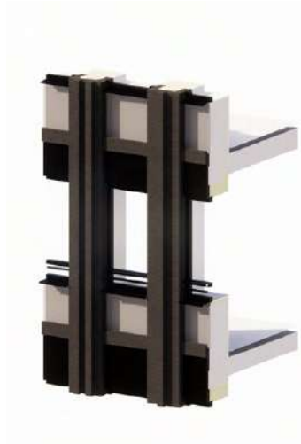
Facade Type 1D - Brickwork
