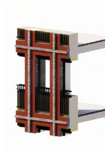
Facade Type 1A - Brickwork
