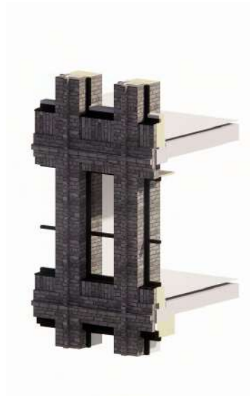
Facade Type 1C - Brickwork
