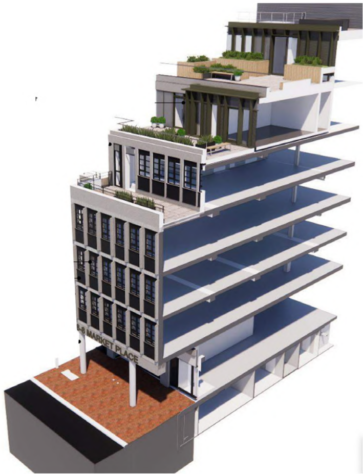
Left: The key elements of the proposals are additional mass adding floors above the existing and a new facade to Market Place
