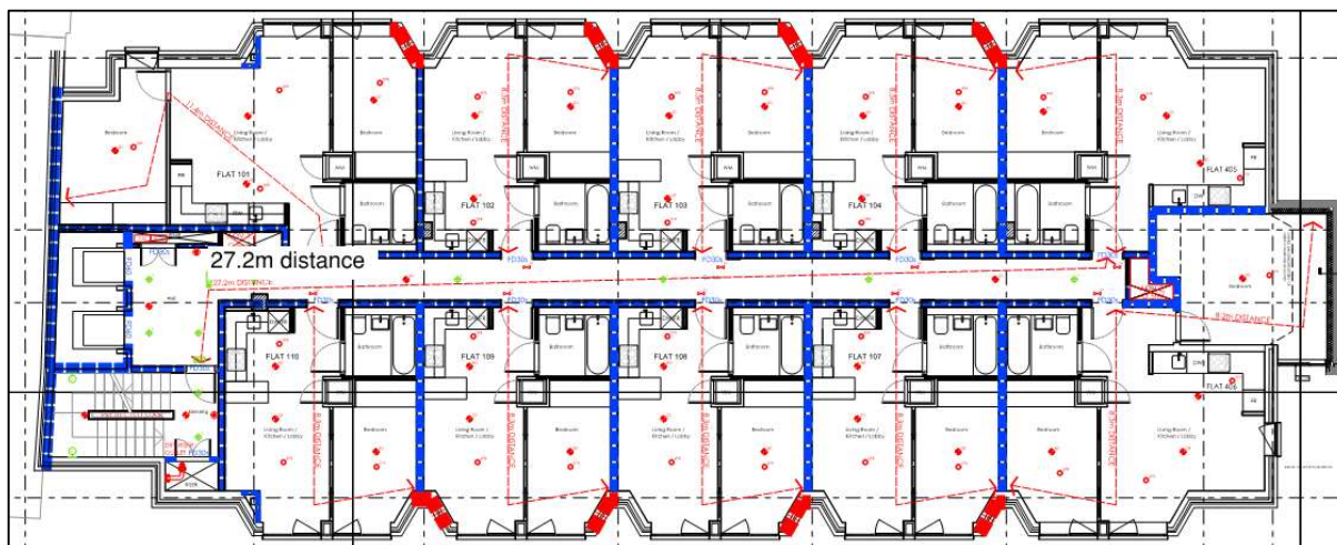
Figure 1 – First to Fourth Floor Corridor Escape Distance
