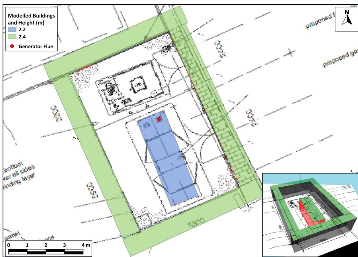
Figure 5: Buildings and Modelled Flue Included in the Model. Inset Shows 3D Image.
