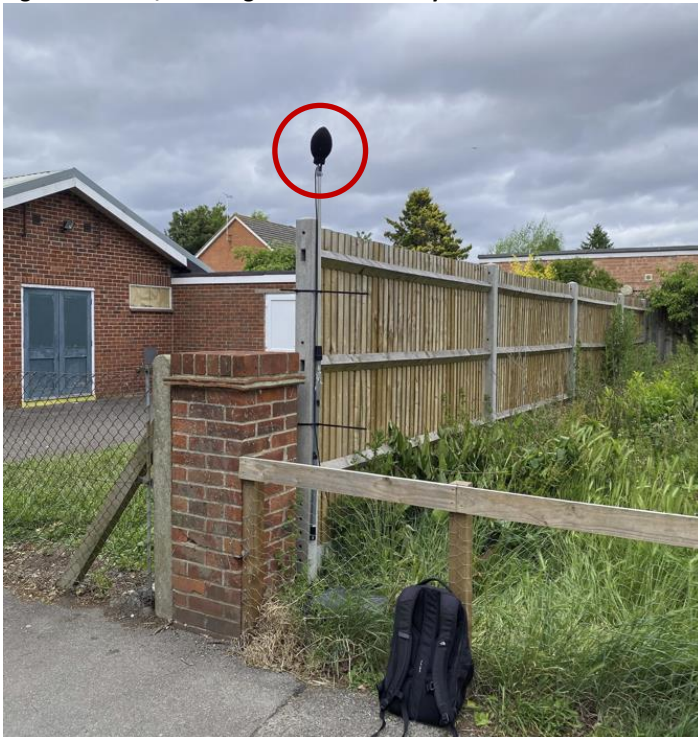
Figure 4.3: Side/Downing Road noise survey location
