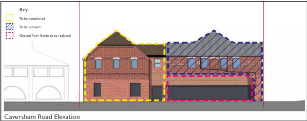
Figure 7 - Retention & Demolition Strategy
