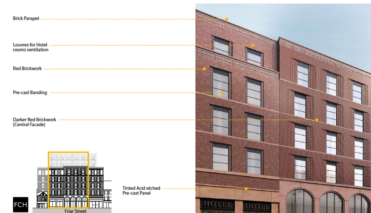
Figure 6.10 Materiality of the front elevation [taken from DAS by FCH Architects]
