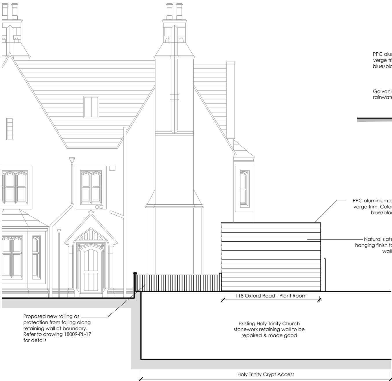
PROPOSED PLANT ROOM SOUTH ELEVATION 1:100
