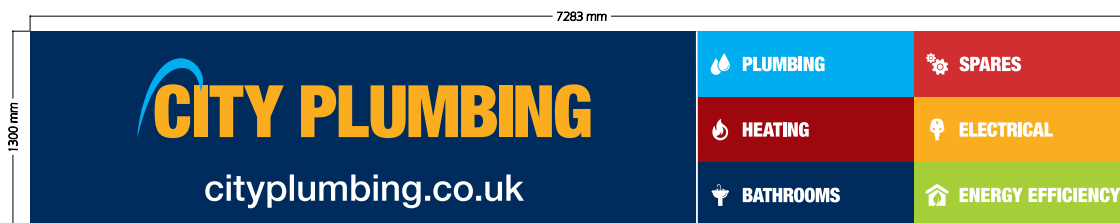
Sign 9 - 1no. Non illuminated flex face sign, box finished PMS 654 Blue, with digitally printed skin. Cap Height = 340mm HTU = 4400mm
