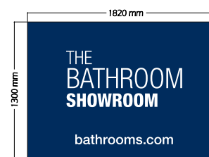
Sign 10 - 1no. Non illuminated flex face sign, box finished PMS 654 Blue, with digitally printed skin. Cap Height = 190mm HTU = 4400mm
