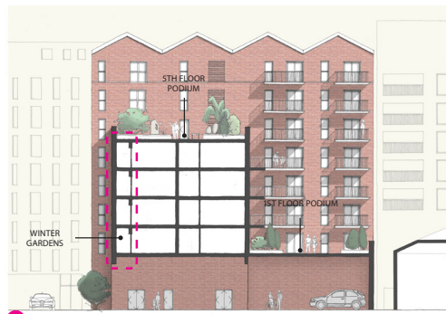
SECTION THROUGH 1ST AND 5TH FLOOR PODIUMS
