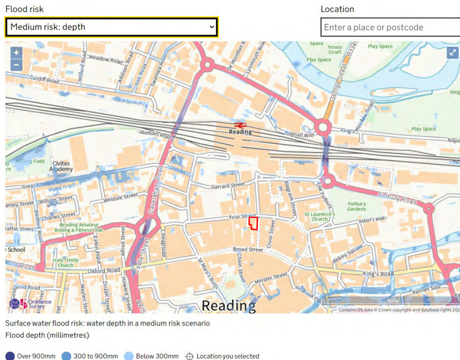
Figure 4.9 Surface water flood map (depth during medium risk flood event) -Source: gov.uk
