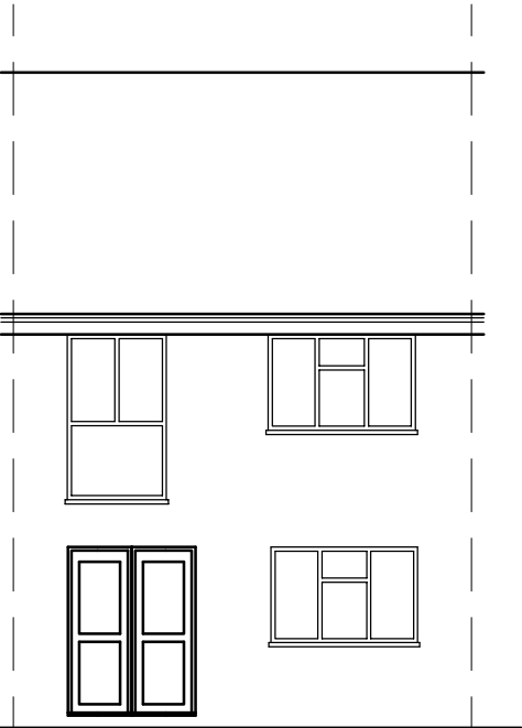
EXISTING REAR ELEVATION
