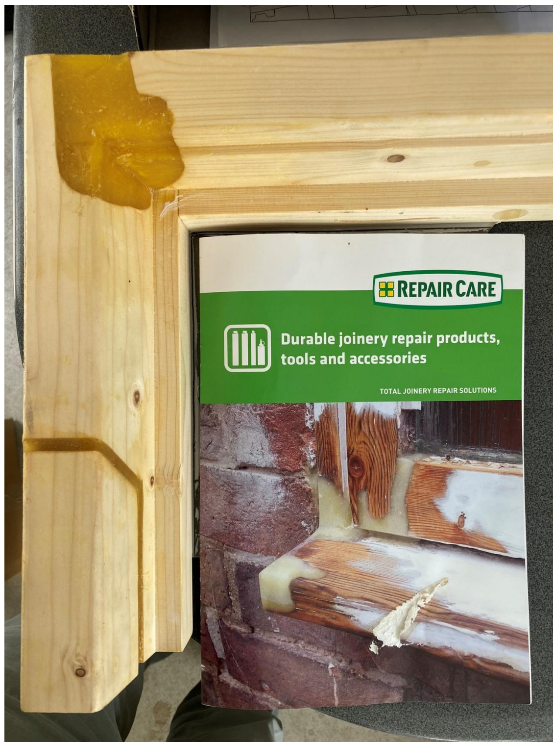
Window frame resin repairs training piece. Maximises retention of original fabric. Thick joints reduce risk of failure at joint
