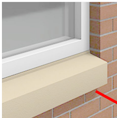
Concrete window cills
