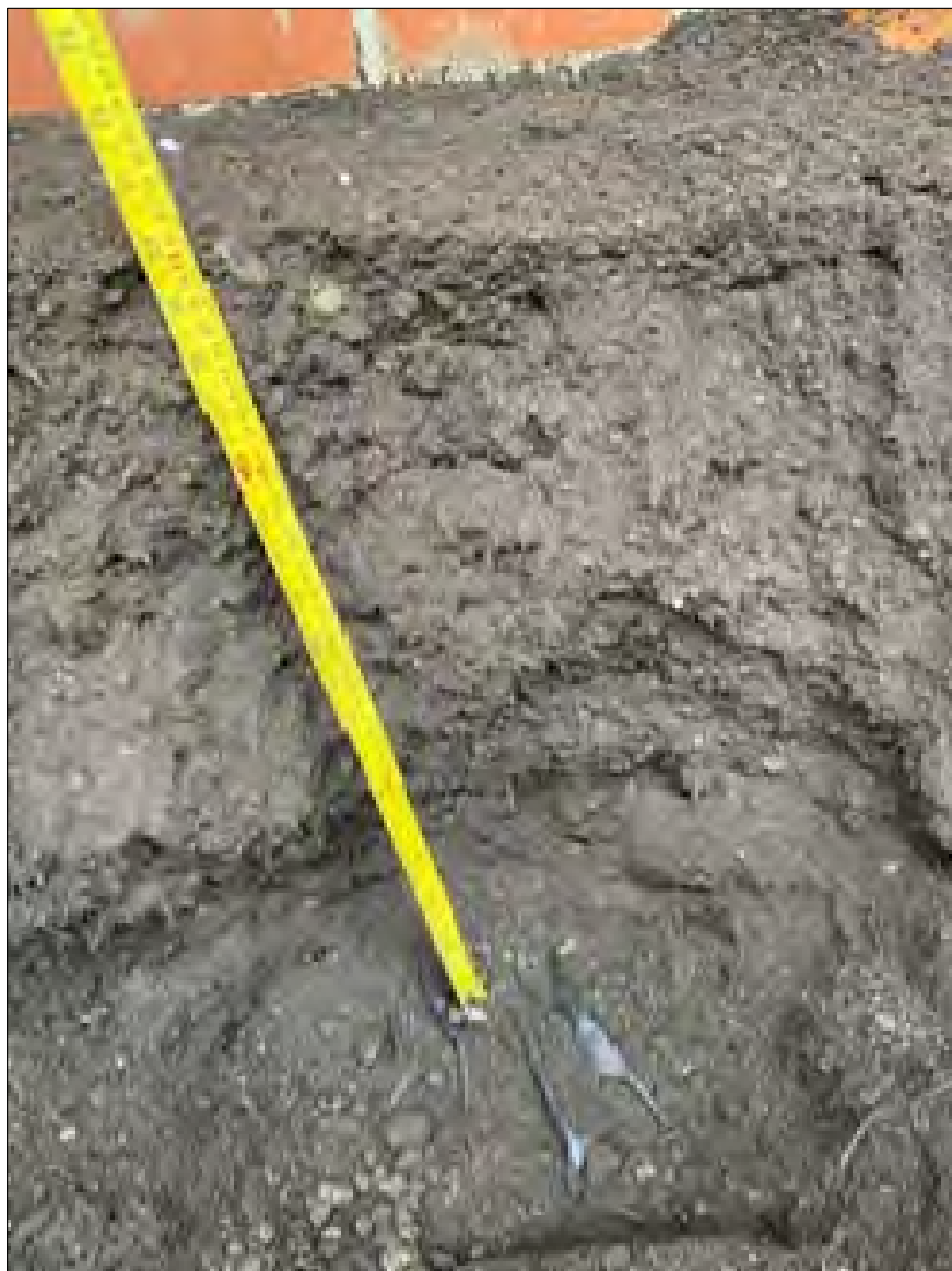
Photo 6: Confirming Clean Cover Thickness and Presence of Geotextile Break Layer within Plot 5
