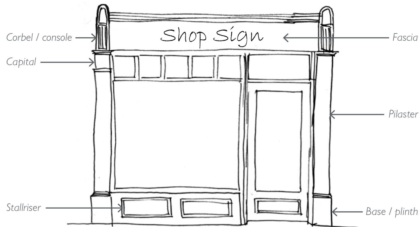
Diagram showing typical features of a single shop front.
