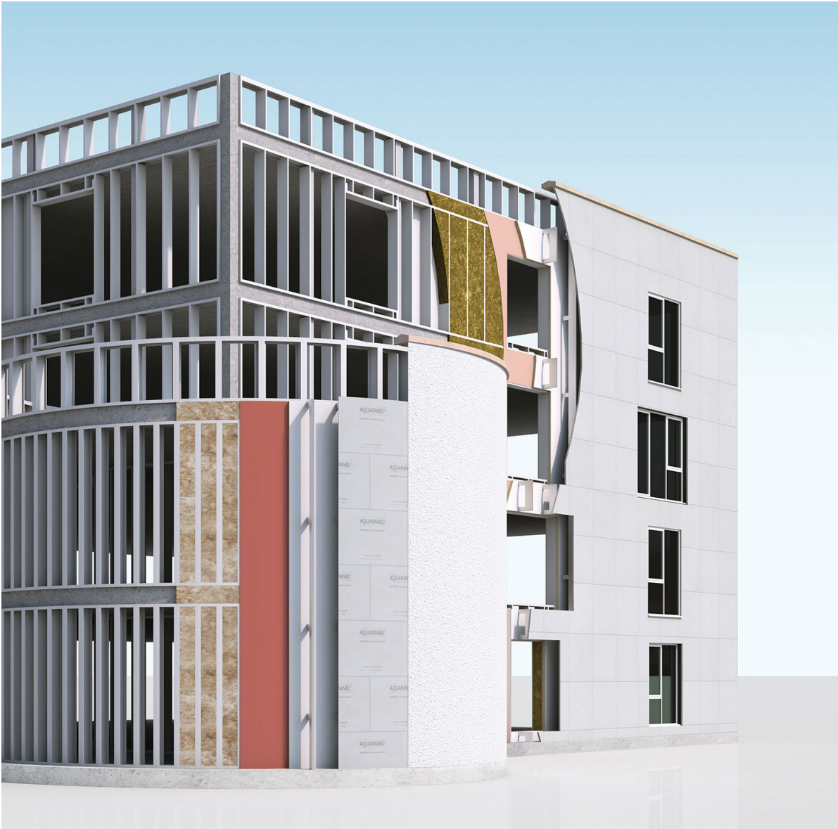
REFERENCE DESIGN - BUILDING CUTAWAY: Rainscreen cladding with high-quality render finish
