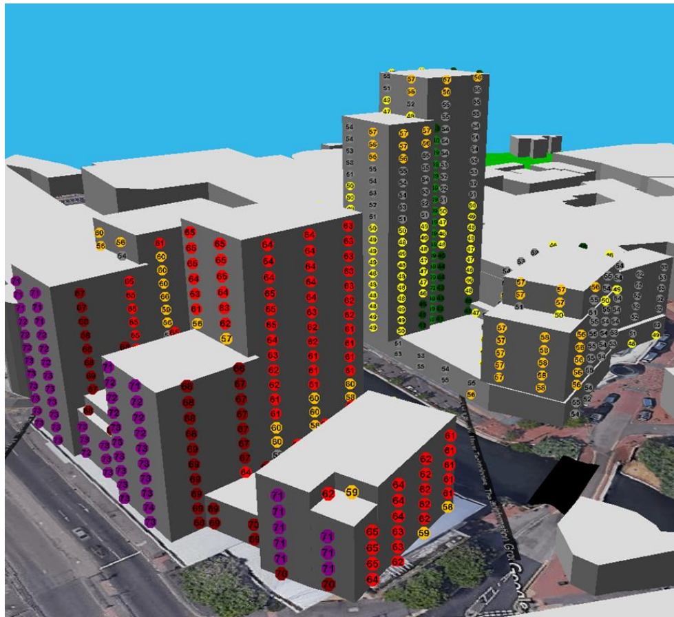
Figure 8 Predicted daytime equivalent continuous noise levels ( L_{Aeq,16hrs} ) at 1m from facades. Southeast view.
