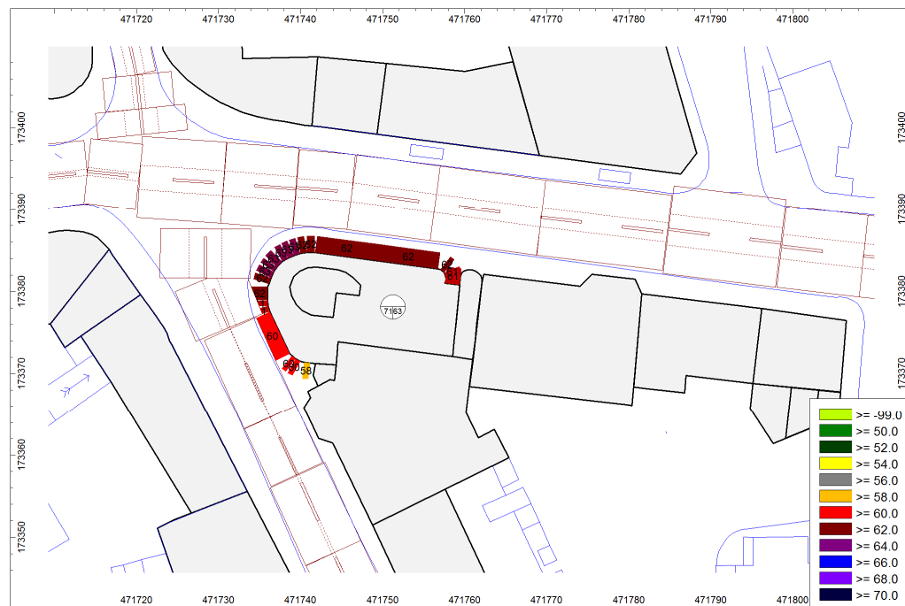
Figure 6: Predicted with-scheme L_{Aeq,8h} noise levels
