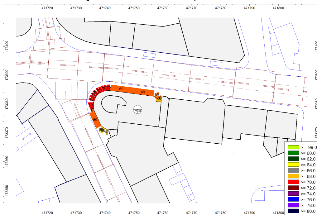
Figure 5: Predicted with-scheme L_{Aeq,16h} noise levels
