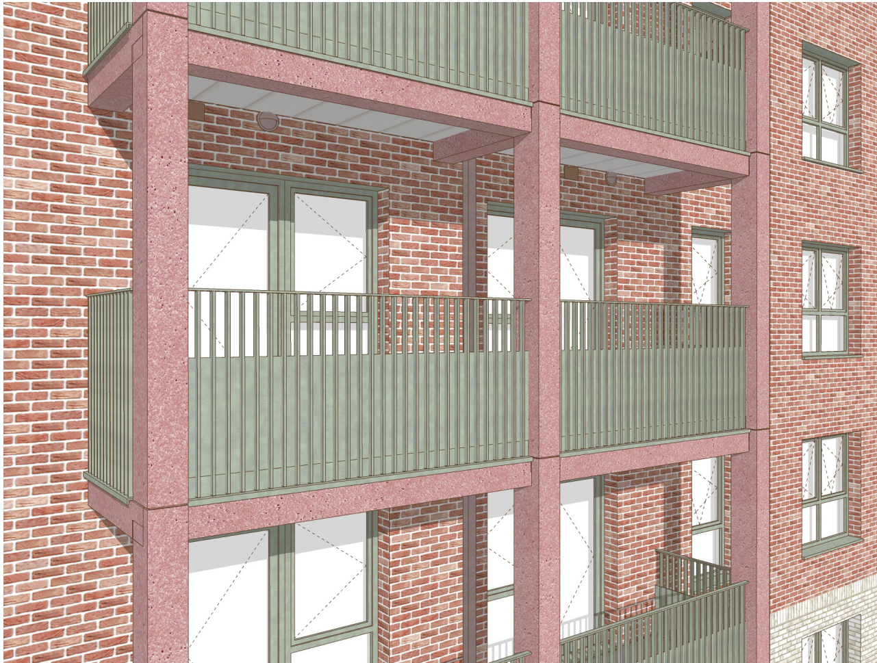
Oblique View - Pre-cast balcony structure
