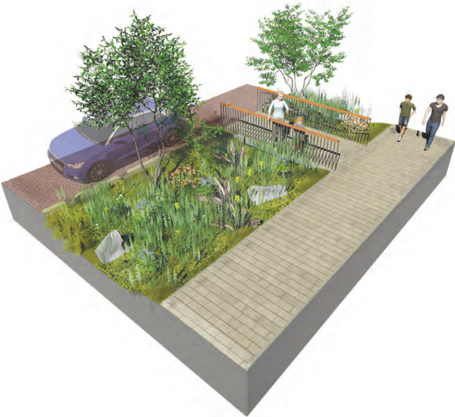
Crossing to dry swale
