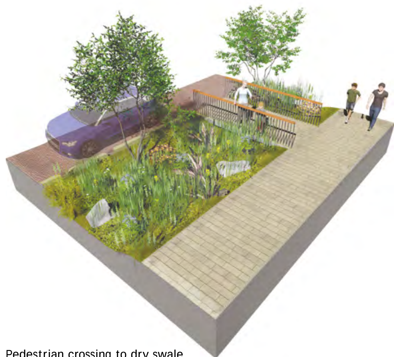
Pedestrian crossing to dry swale
