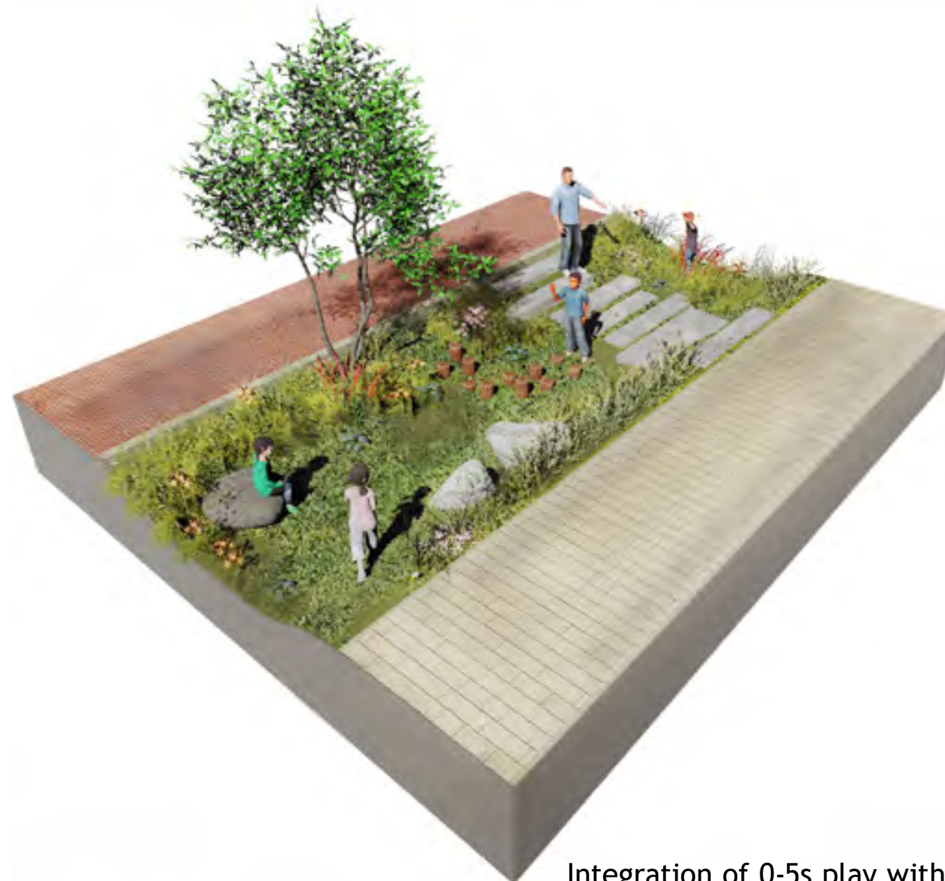
Integration of 0-5s play within dry swale
