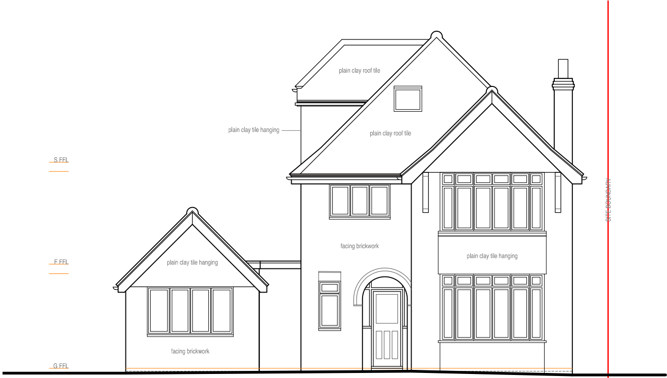
FRONT ELEVATION (NORTH-EAST)
