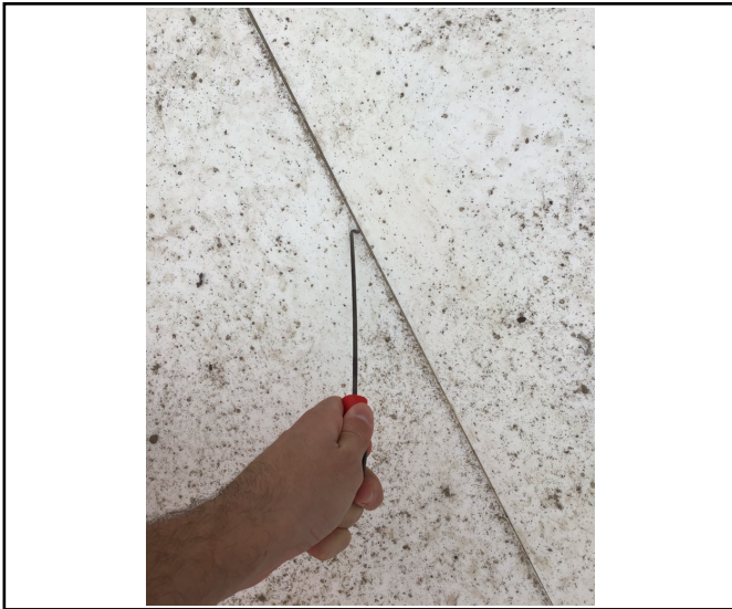
Pick and probe test example.
