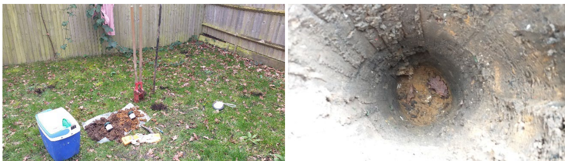
Above left, a trial hole being excavated and sampled. Above right, inside the trial hole
