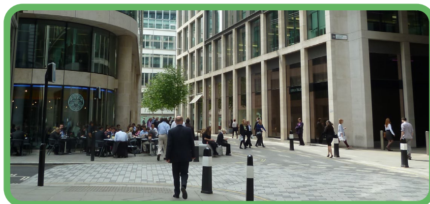
Illustrative examples of pedestrian priority crossing detailing.- Raised Crossing (Copenhagen Crossing), Tactile roadway surfaces, Surfacing change and build-out at crossing.
