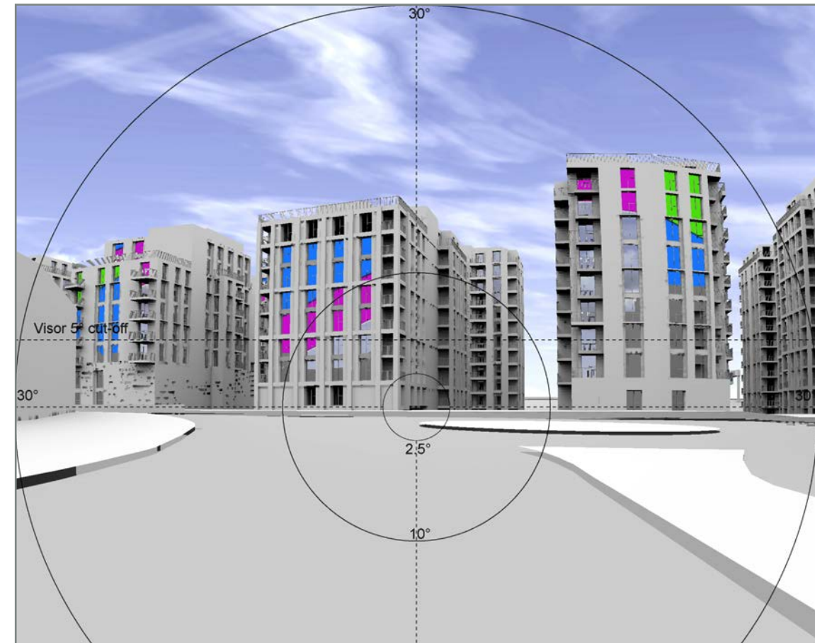
Fig. 95: Solar Glare - MONTHS - Close-up
