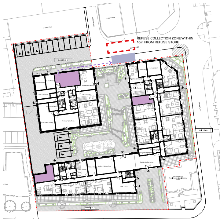
Proposed Ground Floor: Refuse Storage and Loading
