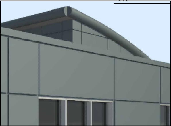
Proposed cladding - Polyester powder coated metal panel system
