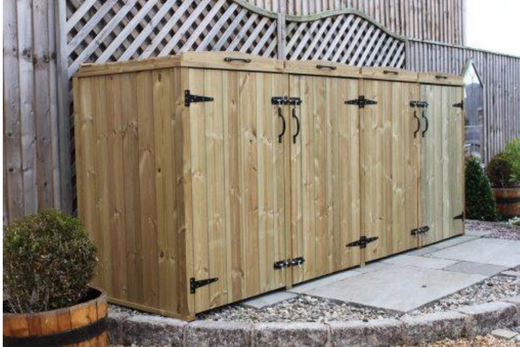
Figure 1 - Bin store to house four 240L bins. The bin store is secure with latched doors and a continuous upstand below to leave no gaps when closed and prevent vermin access.
