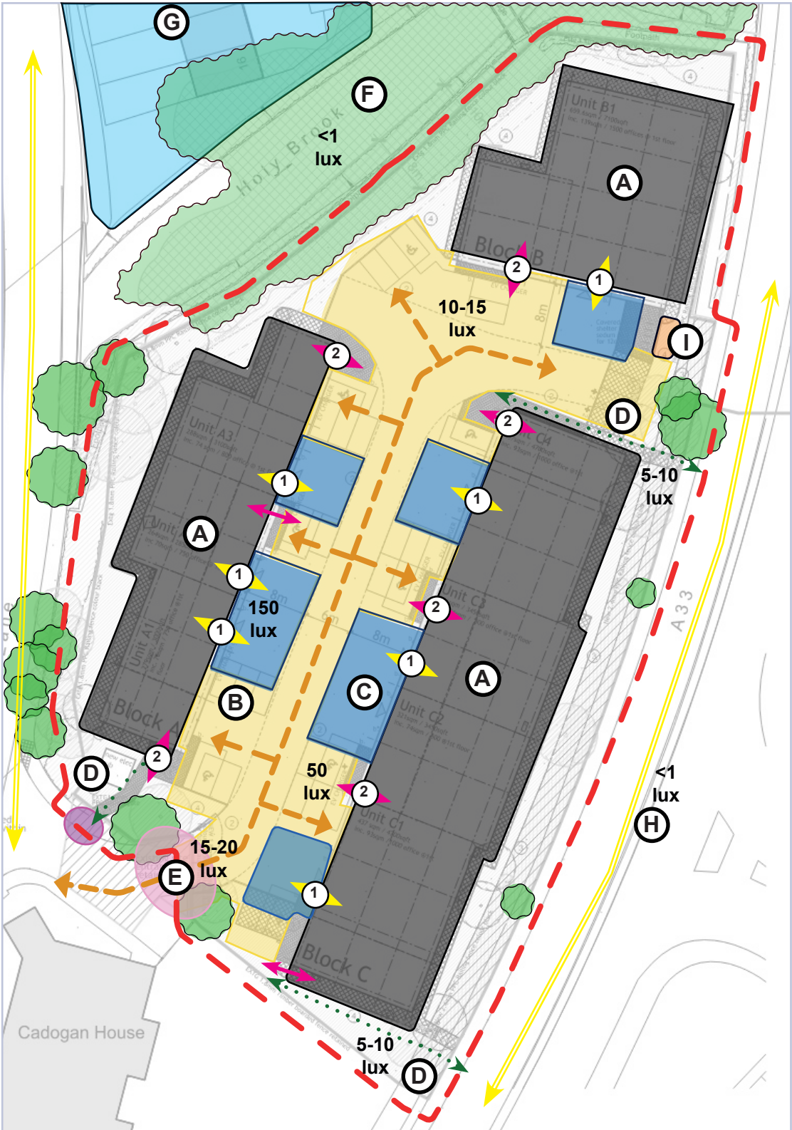
Proposed extension site plan - indicating different lighting zones and access routes.
