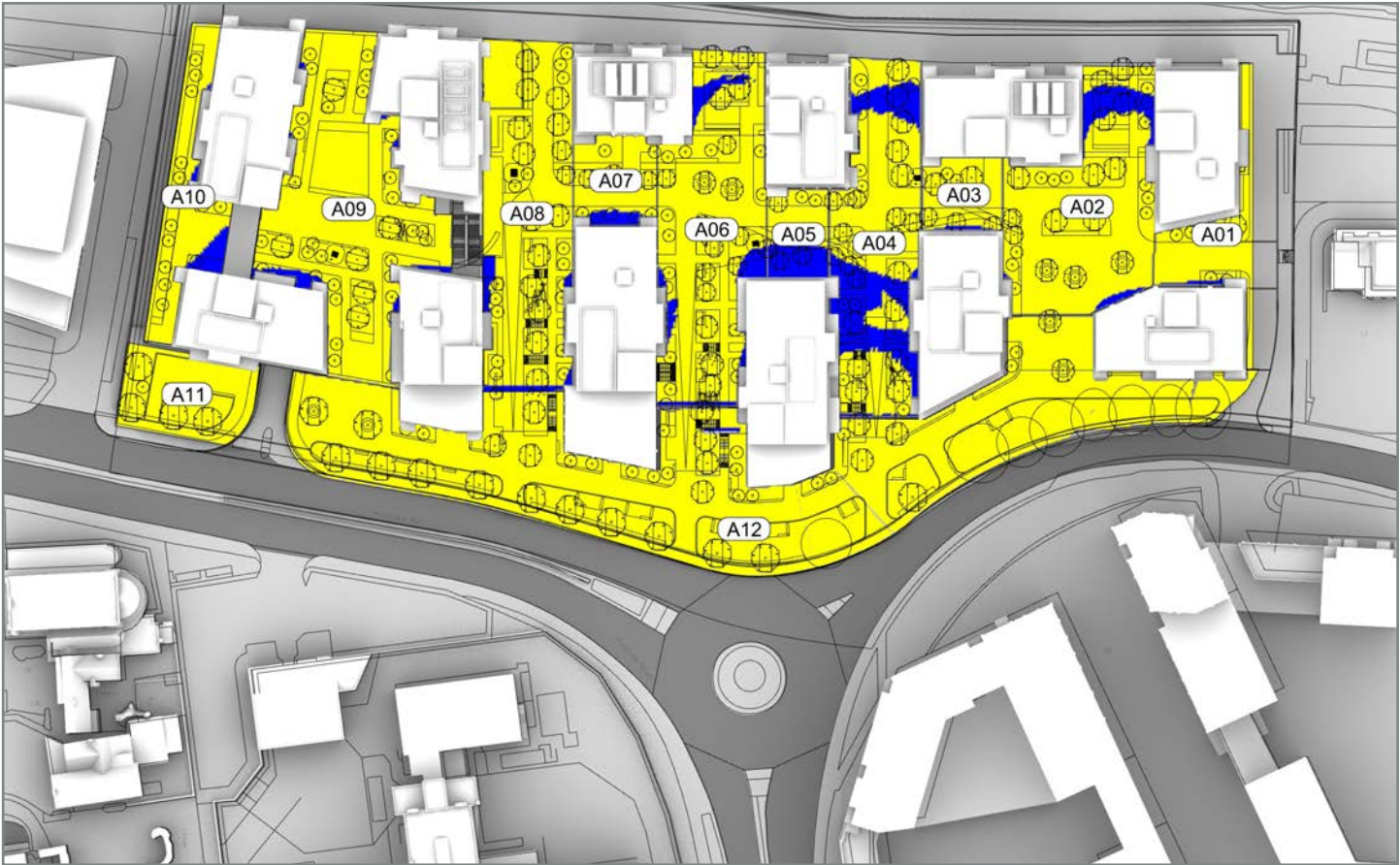
Fig. 4: BRE's Sun on Ground
