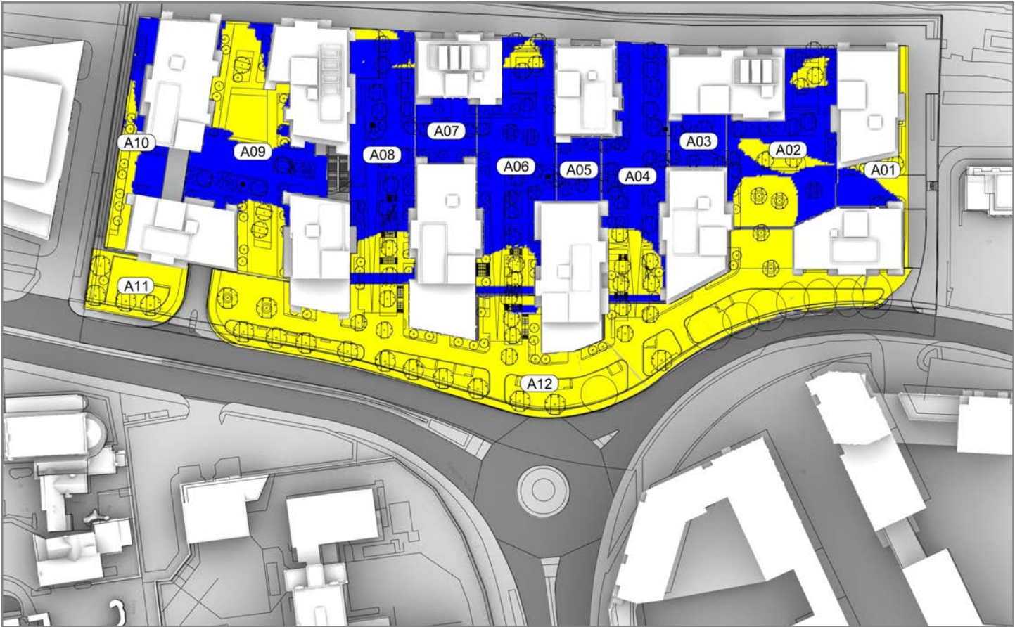
Fig. 2: BRE's Sun on Ground
