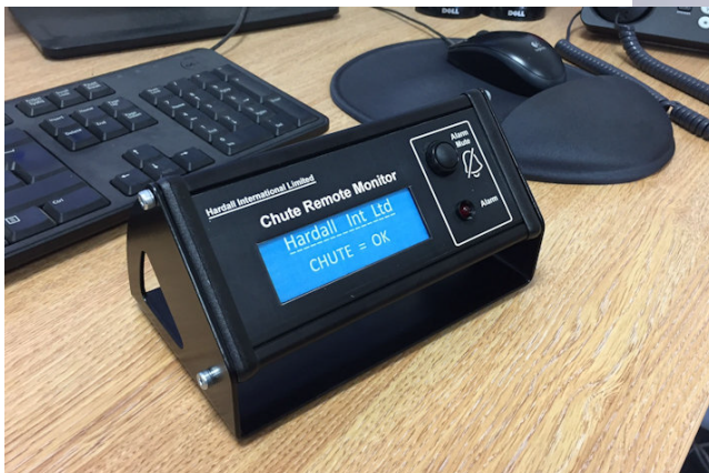
OPTIONAL CHUTE REMOTE MONITOR ( requires CAT 5 Data link )
