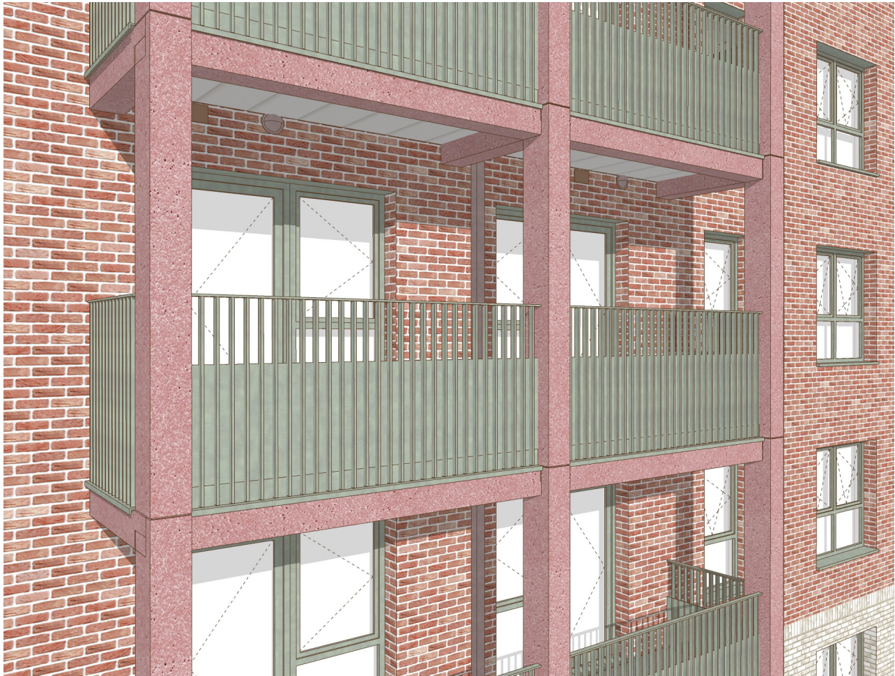
Oblique View - Pre-cast balcony structure
