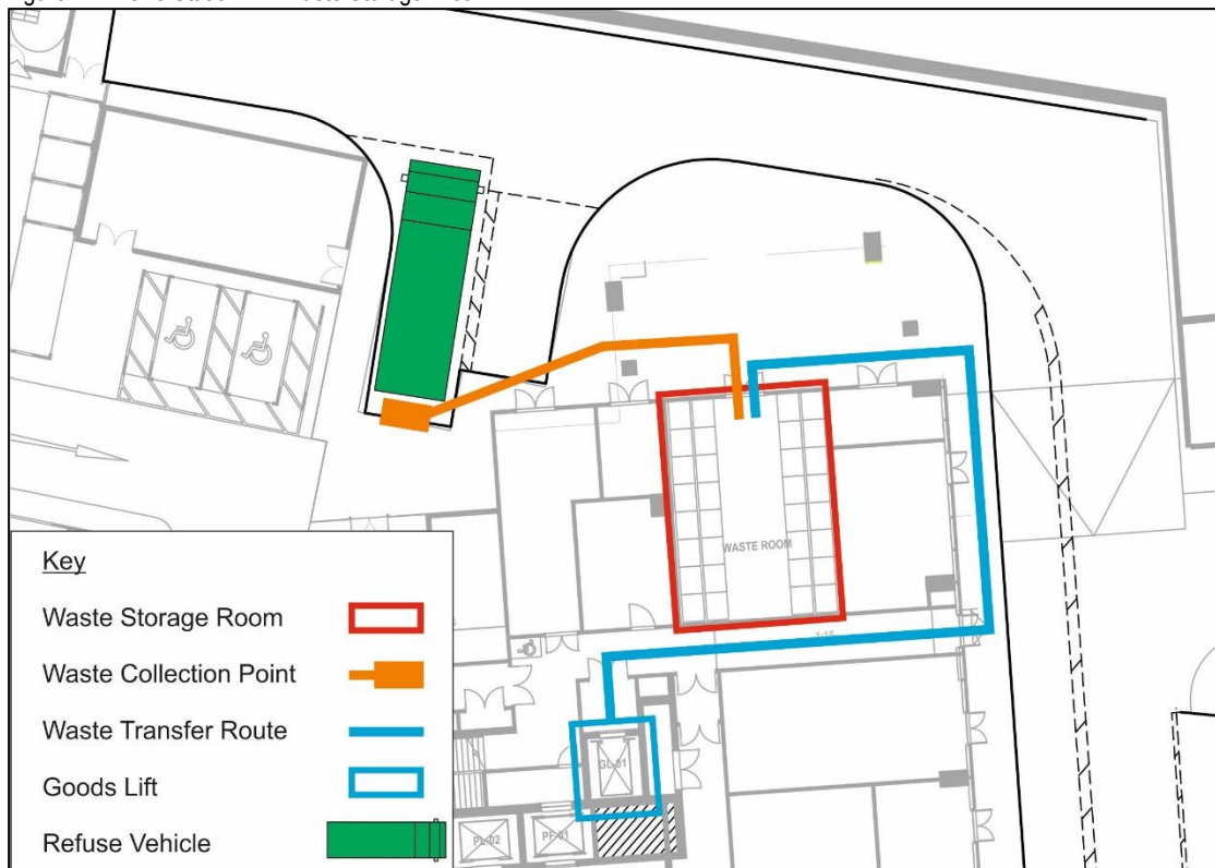
Figure 4.2 – One Station Hill Waste Storage Area
