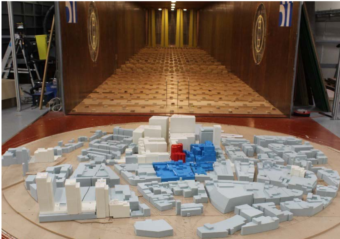
Figure 15: Proposed Development with Cumulative Surrounding Buildings (Configuration 3) - View in the Wind Tunnel (from the south)
