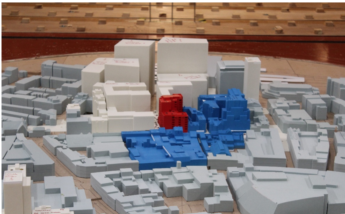
Figure 16: Proposed Development with Cumulative Surrounding Buildings (Configuration 3) - View in the Wind Tunnel (from the south)
