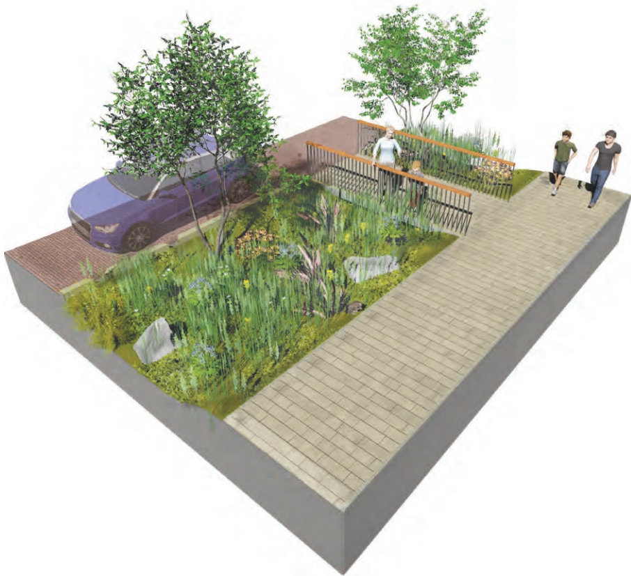
Crossing to dry swale
