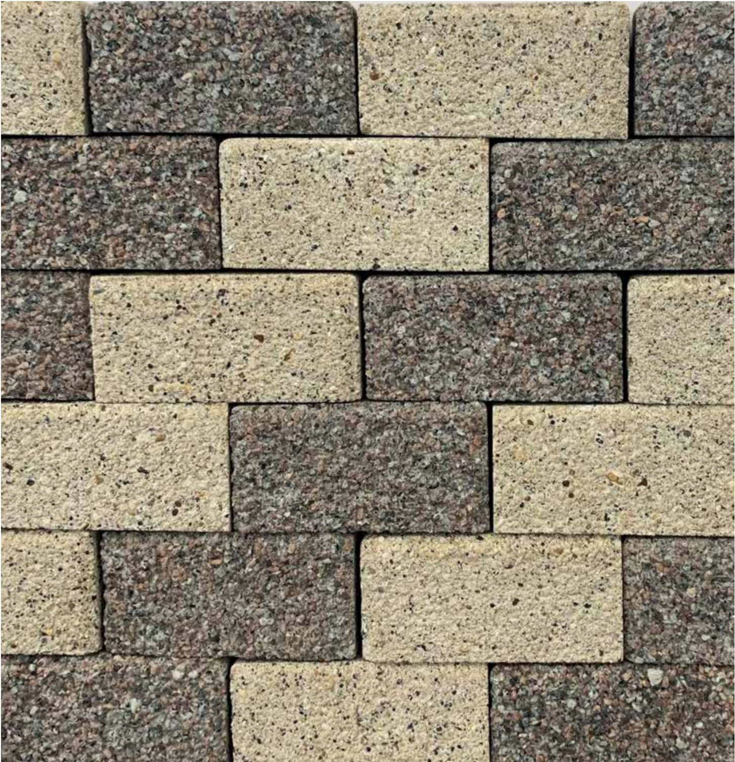
Paving Type 02 - Marshalls Modal 50%Oatmeal, 50% Indian; textured finish. lengths vary, 100mm wide
