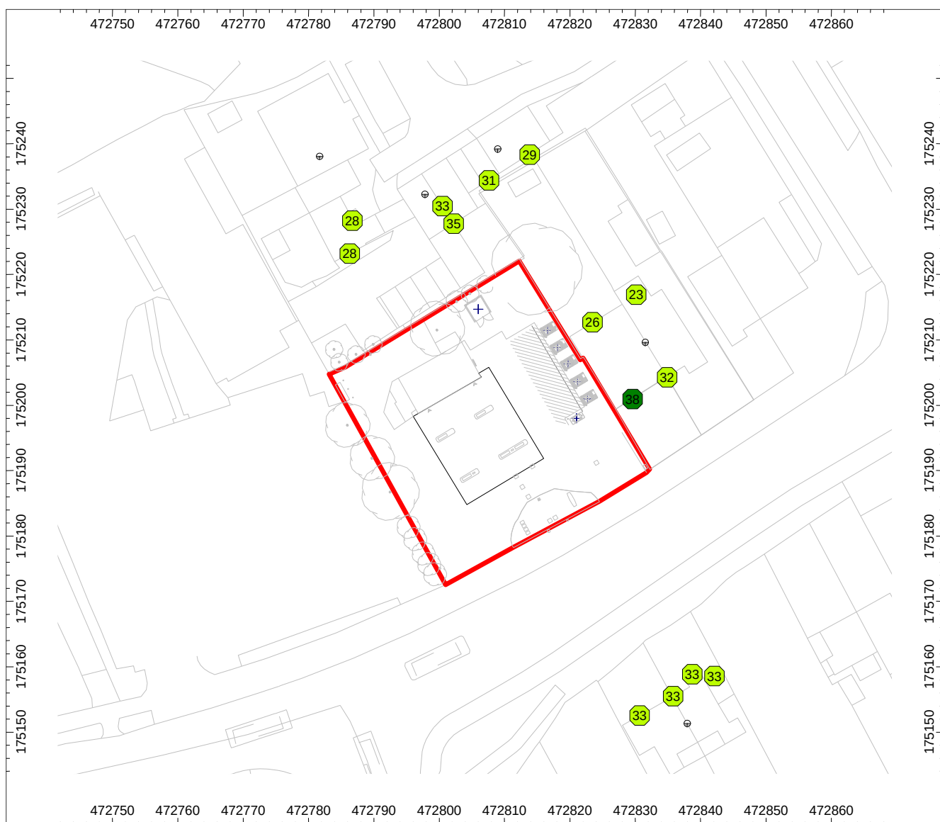
Figure 5-1 Model Outputs of Specific Sound Levels, Highest dB L_{Aeq,T} at Building Façades – All Plant
