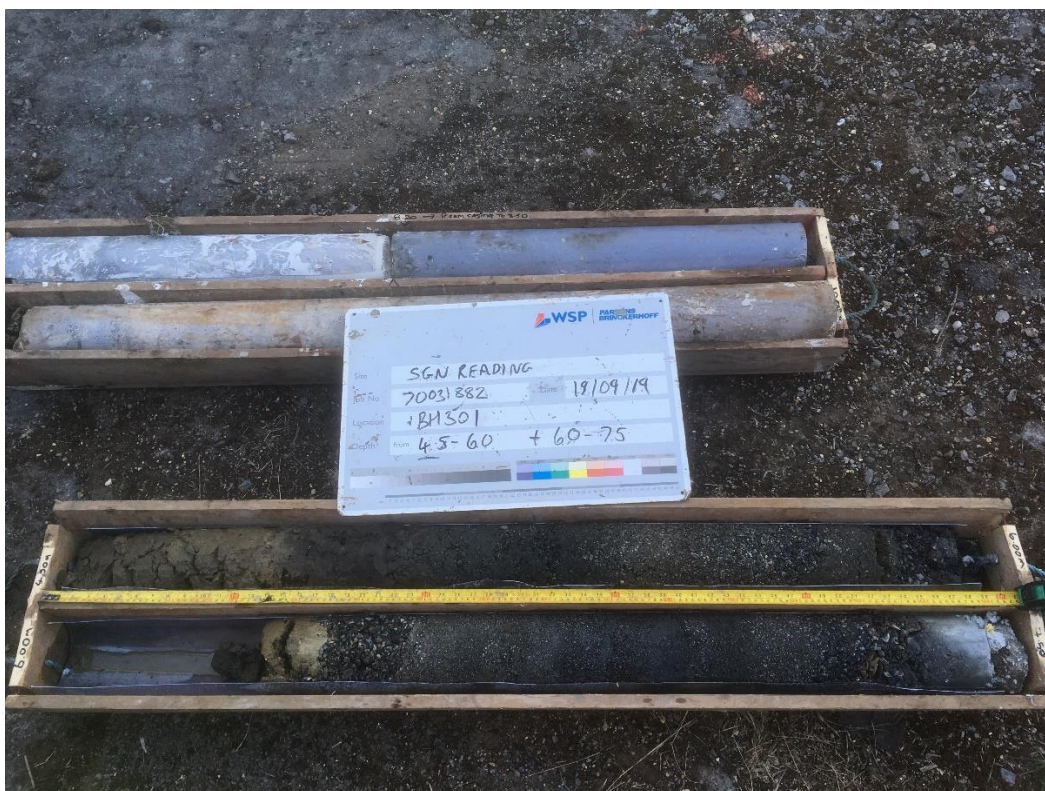
3. BH301: 4.5m to 7.5m bgl
