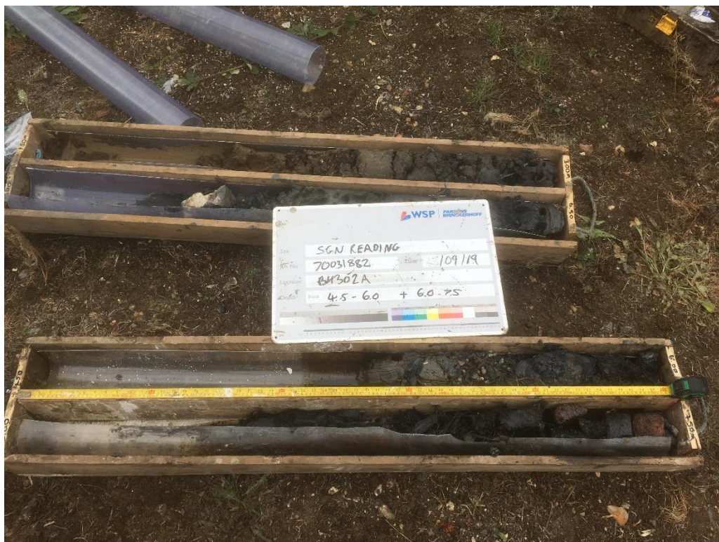
6. BH302A: 4.5m to 7.5m bgl
