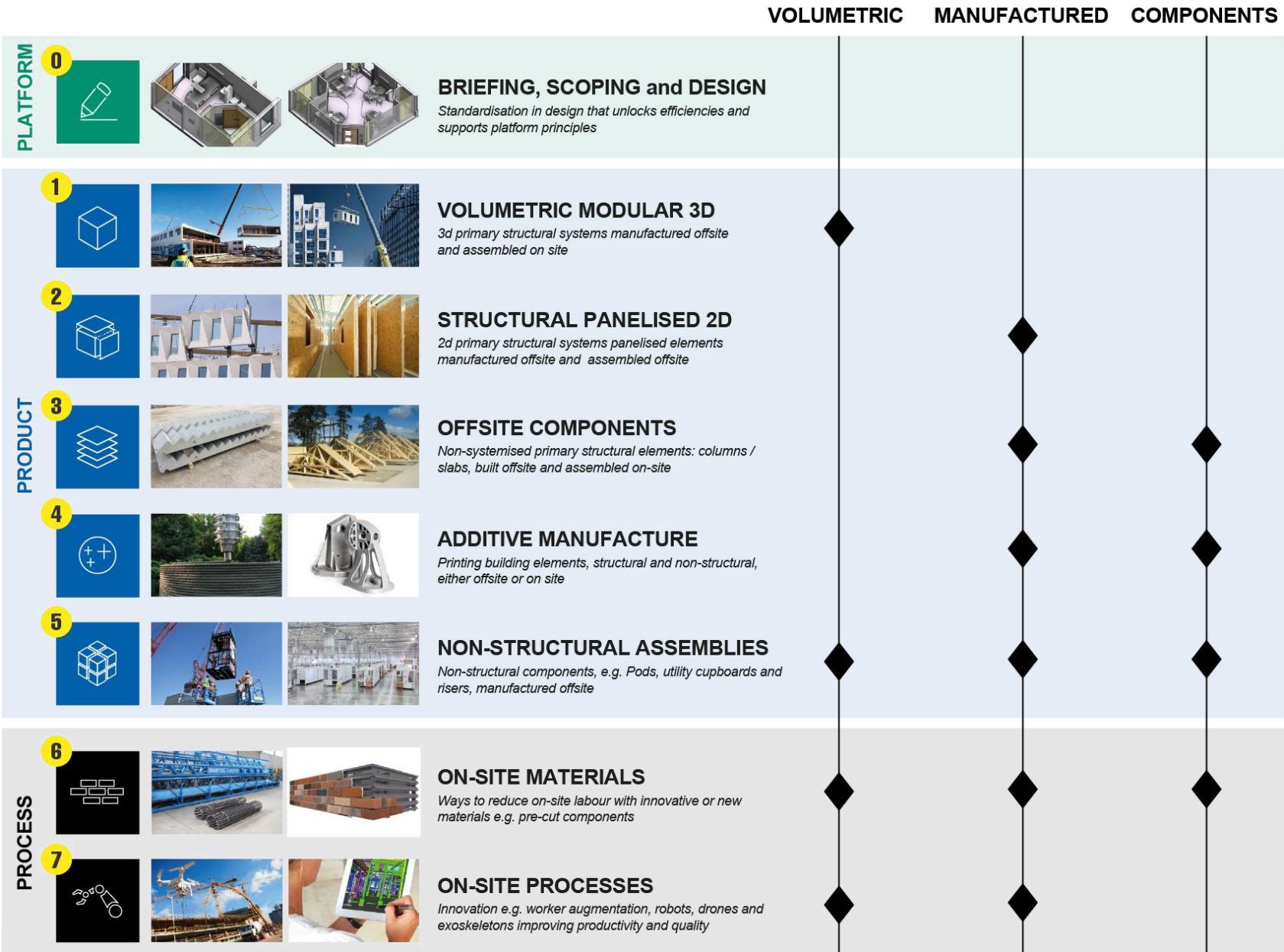
7 + 1 Categories of MMC (Adapted from MHCLG Definition Framework)
