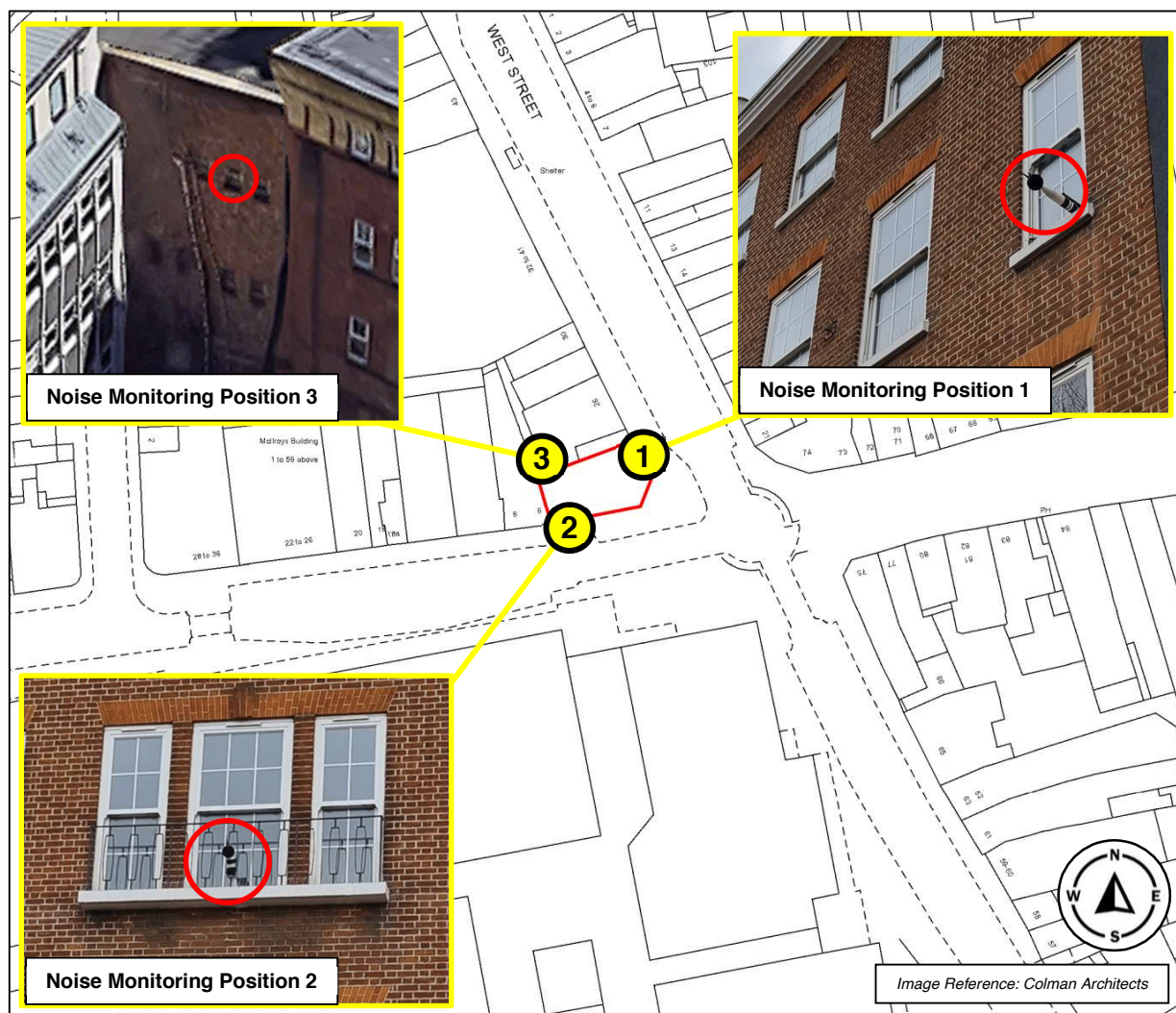
Figure 3 Noise survey measurement locations
